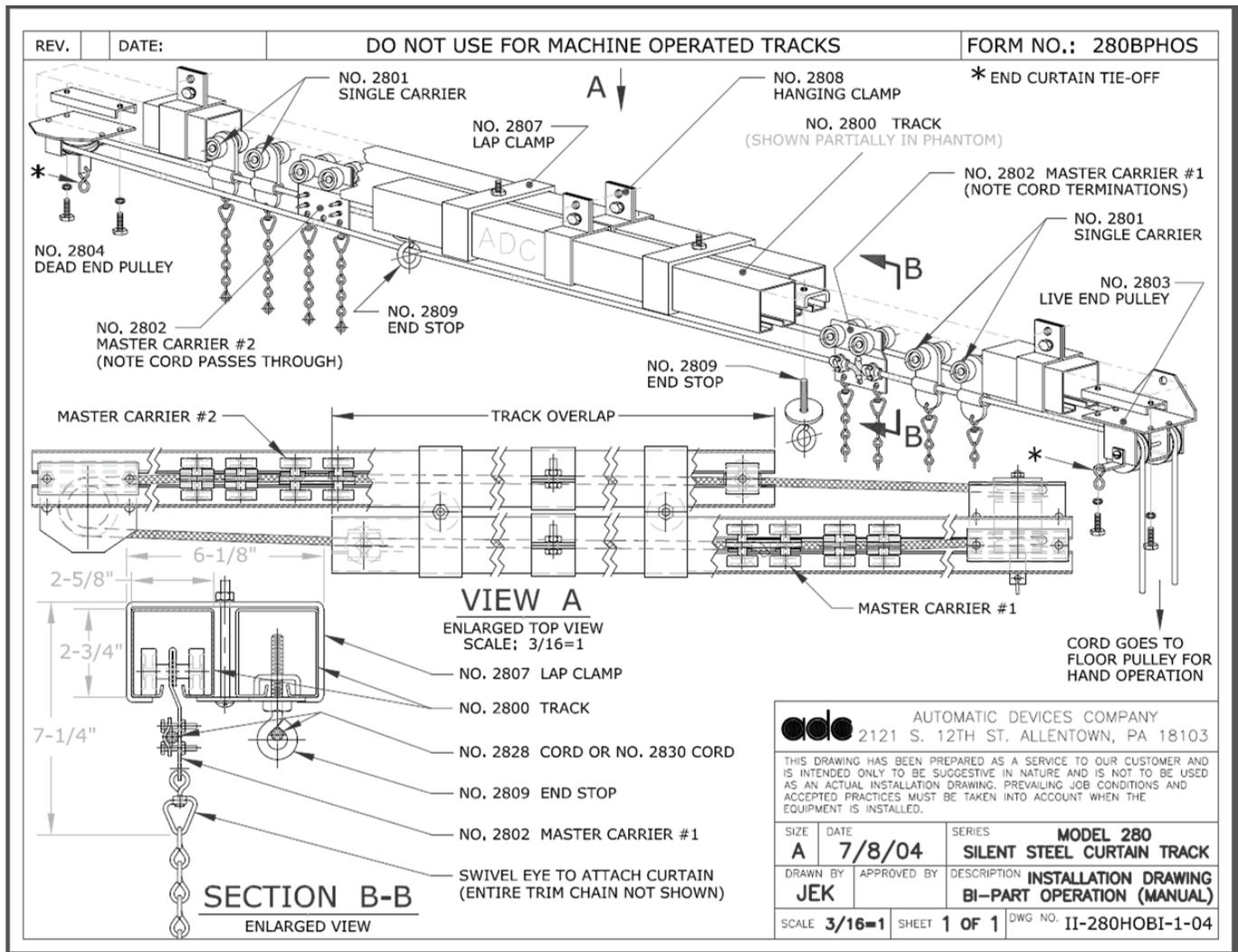
Note diagram shows overlapping tracks, it is also possible to use overlapping master carriers and a single track
