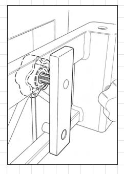
Guardrails are modular and do not interconnect. Units comprise the guardrail, two backplates and two hand knobs. Guardrails are fixed as follows:
