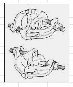
Stages built over four feet high must be cross-braced with horizontal and diagonal lengths of 1½ Schedule 40 pipe for stability and safe use. Bracing must be secured with standard fixed (two way) and swivel clips. All bracing components are available from Steeldeck, Inc.
